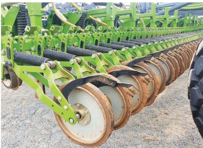
The Simons' Boss TX45 parallelogram unit is followed by a press wheel system.
