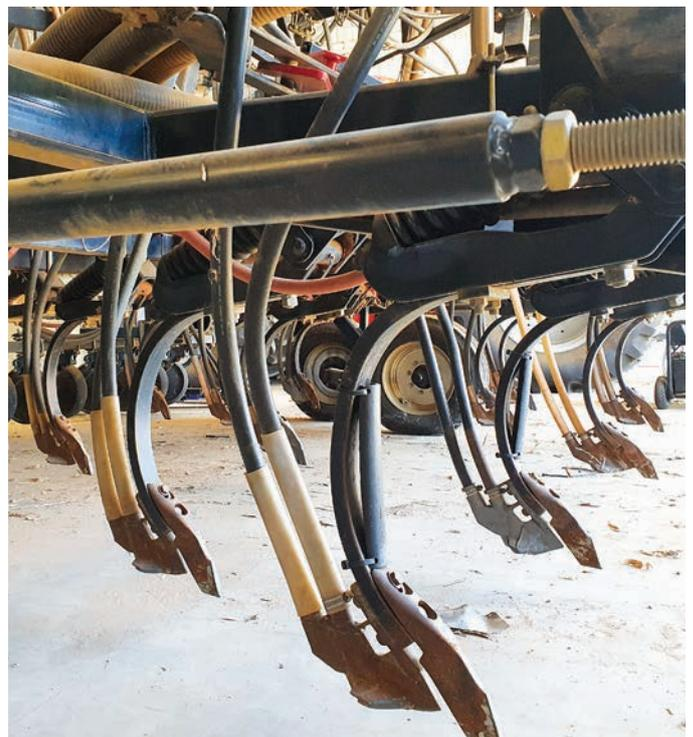
The seeder bar with paired-row ribbon points and root boots has improved seed and fertiliser placement.
