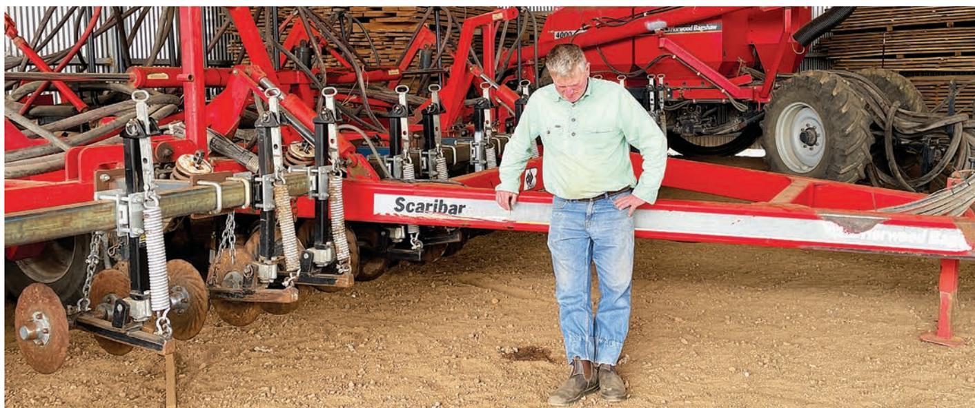
One change Stuart Robinson made to the seeder was to add coulters to aid with seeding through retained stubbles. They built their own toolbar and put Knuckey coulters across the front.
