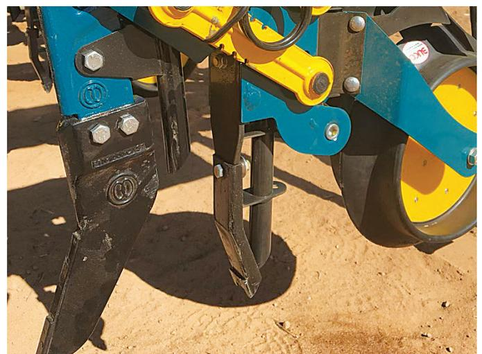
Row unit set-up showing independent press wheel regulated seed banding boot, opener.
